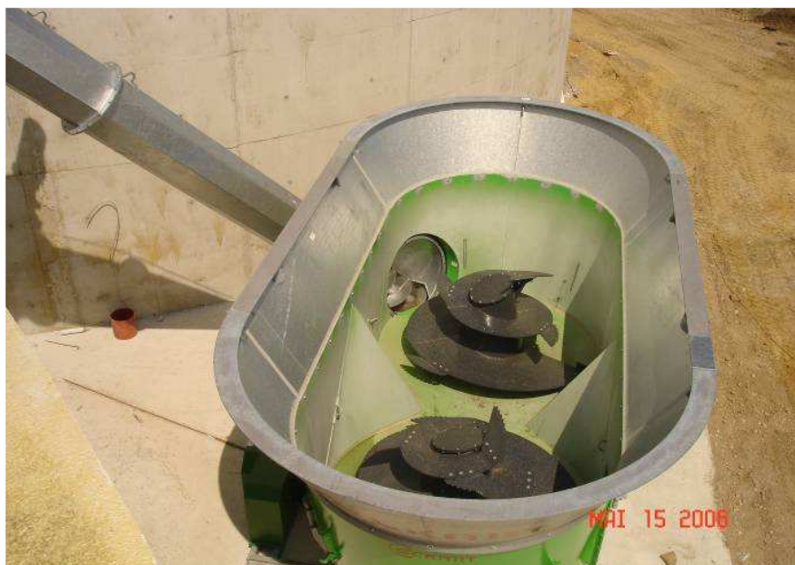
Figure 7.14 Feed-in system for silage (AGRINZ 2006)
